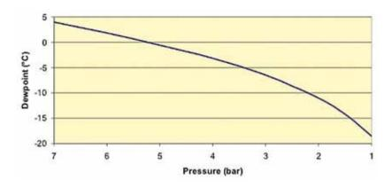
a dew point reading of  $+4^{\circ}\text{C}$  might give the impression that the system is operating correctly. However, when pressure dependence is taken into account, the actual dew point at the dryer is only  $+6^{\circ}\text{C}$ . This example shows that the best dew point measurement location is directly on the dryer outlet.
