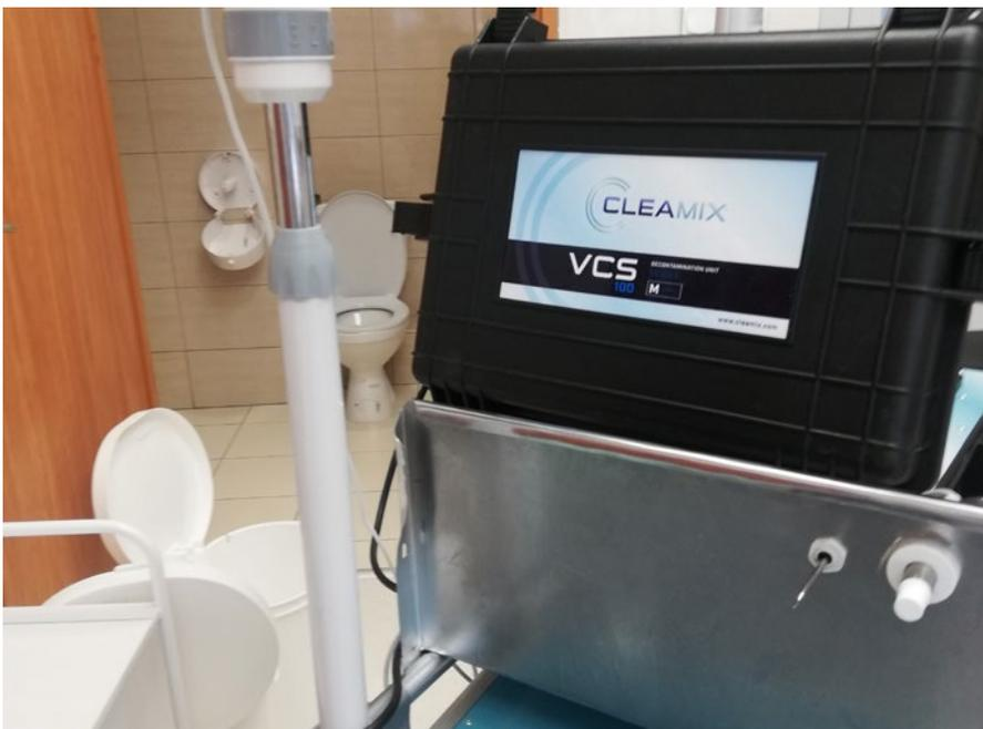
One of the vapor generators Iacobus uses is the Cleamix portable vapor generator, which comes equipped with Vaisala’s HPP270 vaporized hydrogen peroxide probe. The probes provide various parameter measurements, including: hydrogen peroxide vapor, temperature, and humidity as relative saturation and relative humidity, dew point, and vapor pressure. The HPP270 probes can be integrated with a vapor generator or control system to control processes.
