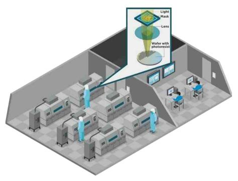
Precision air conditioning and wafer stepper process capacity can be significantly enhanced with accurate and stable measurement of air pressure, temperature, and humidity.
