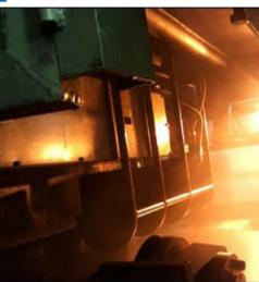
1 LaserSpeed measuring the continuous length of slab casters and making cuts with ±0.03% or better precision.
