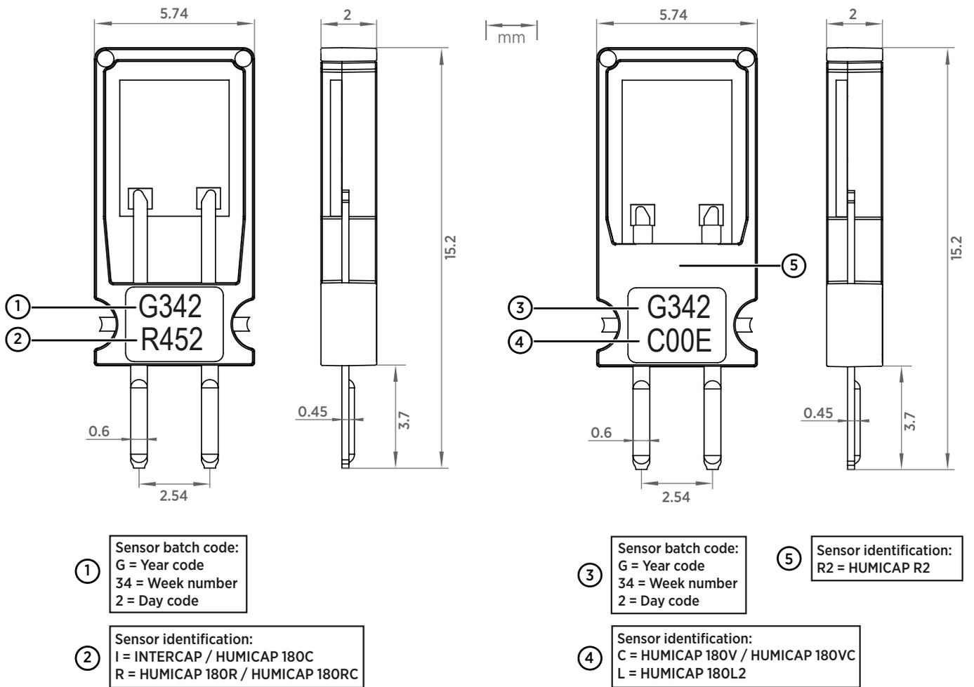
Type C (left) and type D (right) encapsulation dimensions
