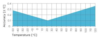
HMP80L temperature measurement accuracy over full range
