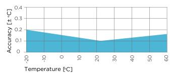
HMP80N temperature measurement accuracy over full range
