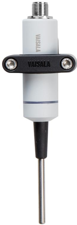
Vaisala HUMICAP® Humidity and Temperature Probe HMP1 is designed for ambient measurement in indoor spaces. Its probe head and body are integrated into a single unit with no cable between them. HMP1 can be directly connected to Indigo200 series transmitters to form a single wall-mounted unit.
