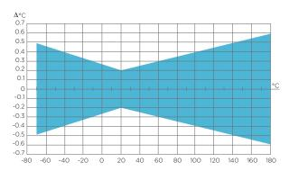
Temperature measurement accuracy over temperature
