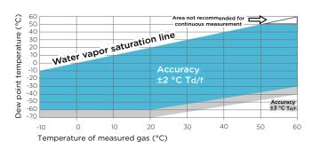
Dew point accuracy vs. measurement conditions (DMP80B)
