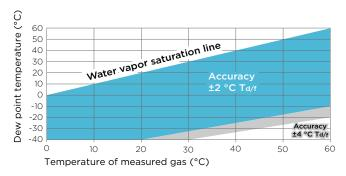
Dew point accuracy vs. measurement conditions (DMP80A)
