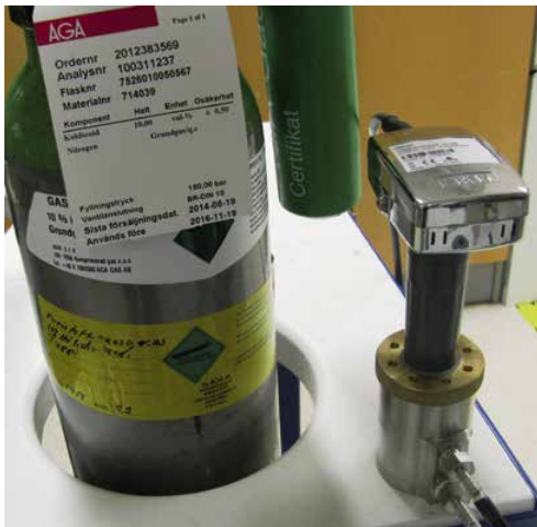
Figure 4. Gas cylinder and test cell used for the CO 2 measurement (left). Example of the recorded CO 2 readings at the four test concentrations (right).
