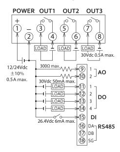
Note: • Terminal SG (for RS-485) is connected to terminal 2 in the terminal block inside the unit.
