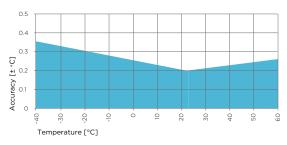
HMP1 temperature measurement accuracy over full range
